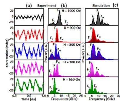
Spin waves excited in a single elliptical Co nanomagnet of major axis 190 nm and minor axis 186 nm excited by a surface acoustic wave (SAW) in the underlying piezoelectric substrate. The SAW is generated by ultrashort (100 fs) laser
