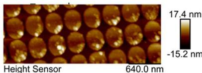
Atomic force micrograph of arrays of dipole-coupled nanomagnets of lateral dimension ~ 200 nm fabricated on a piezoelectric PMN-PT substrate in the speaker's lab that emulated simulated annealing when excited by time-varying strain pulses..
